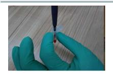
6.Press start, drop 3ul sample to the right position of cartridge and push it back into the instrument
