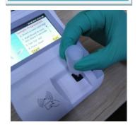
4.After reading the card, press "Test" button and the screen will show as below
